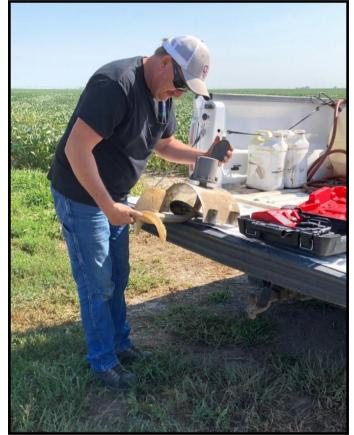
*Jauken inspects* a flow meter that isn't working properly before deciding whether he can fix the problem or to replace the meter altogether.
